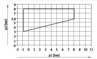
For valves in width 14 mm with code for position function 1-32: MS, NS, KS, HS, DS  $\,$
