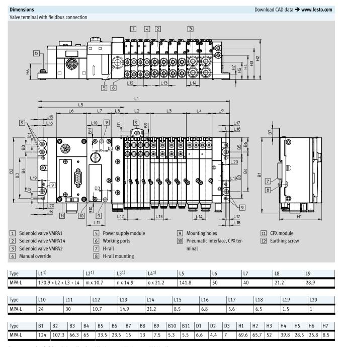
$<sup>1) \\ \\</sup> m, \\ n, \\ o = number of \\ sub-bases/valve \\ positions \\ \\ (m = width \\ 10 \\ mm, \\ n = width \\ 14 \\ mm, \\ o = width \\ 20 \\ mm) \\ \\ mn = width \\ mn \\ o = width \\ o = widt$
