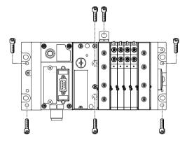
The MPA-L valve terminal is screwed onto the mounting surface using four M4 and two M6 screws or using six M6 screws. The mounting holes are
