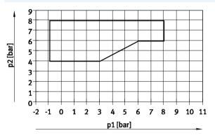
For valves in width 20 mm with code for position function 1-32: MS, NS, KS, HS, DS  $\,$
