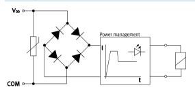
Each solenoid coil is protected with a spark arresting protective circuit as well as against polarity reversal. All valve types are additionally equipped with integrated current reduction.
