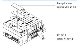
A holder VMPAL-ST-AP-10 (Part No. 561109) with inscription labels (Part No. 18576, IBS-6x10) can be mounted on each sub-base for labelling the valves.
